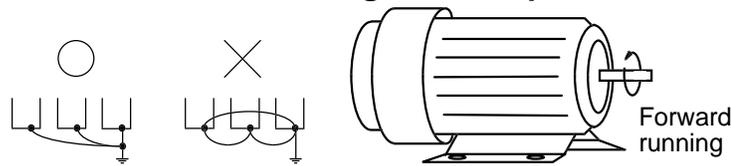
8. When the AC drive output terminals U/T1, V/T2, and W/T3 are connected to the motor terminals U, V, and W, respectively, the motor will rotate counterclockwise (as viewed from the shaft ends of the motor) when a forward operation command is received. To reverse the direction of motor rotation, switch over any of the two motor leads.
